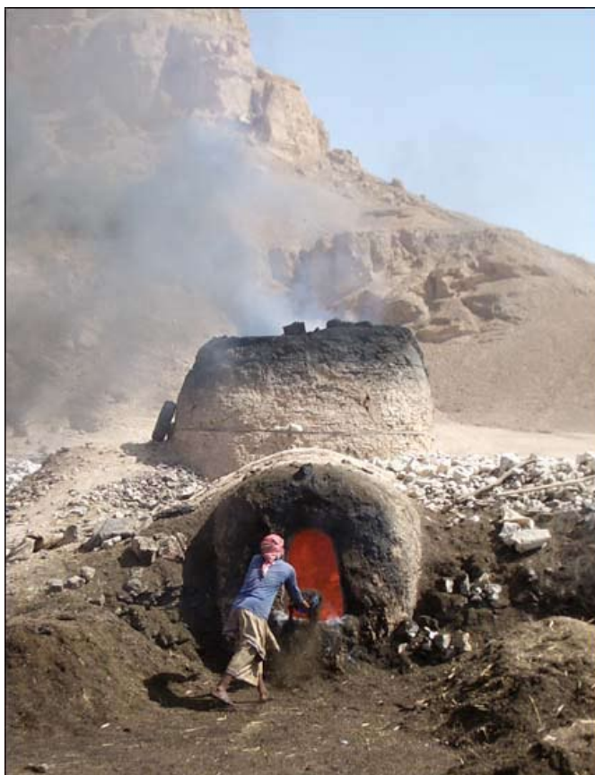
Fig. 19. Oven for burning limestone in the process of creating nurāh plaster. http://ilovecob.com/ashan/mudmasters/mm25.htm .
