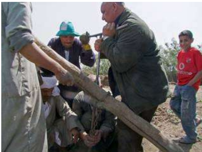
Extracting a 'stuck' drill core at Kom Usim
